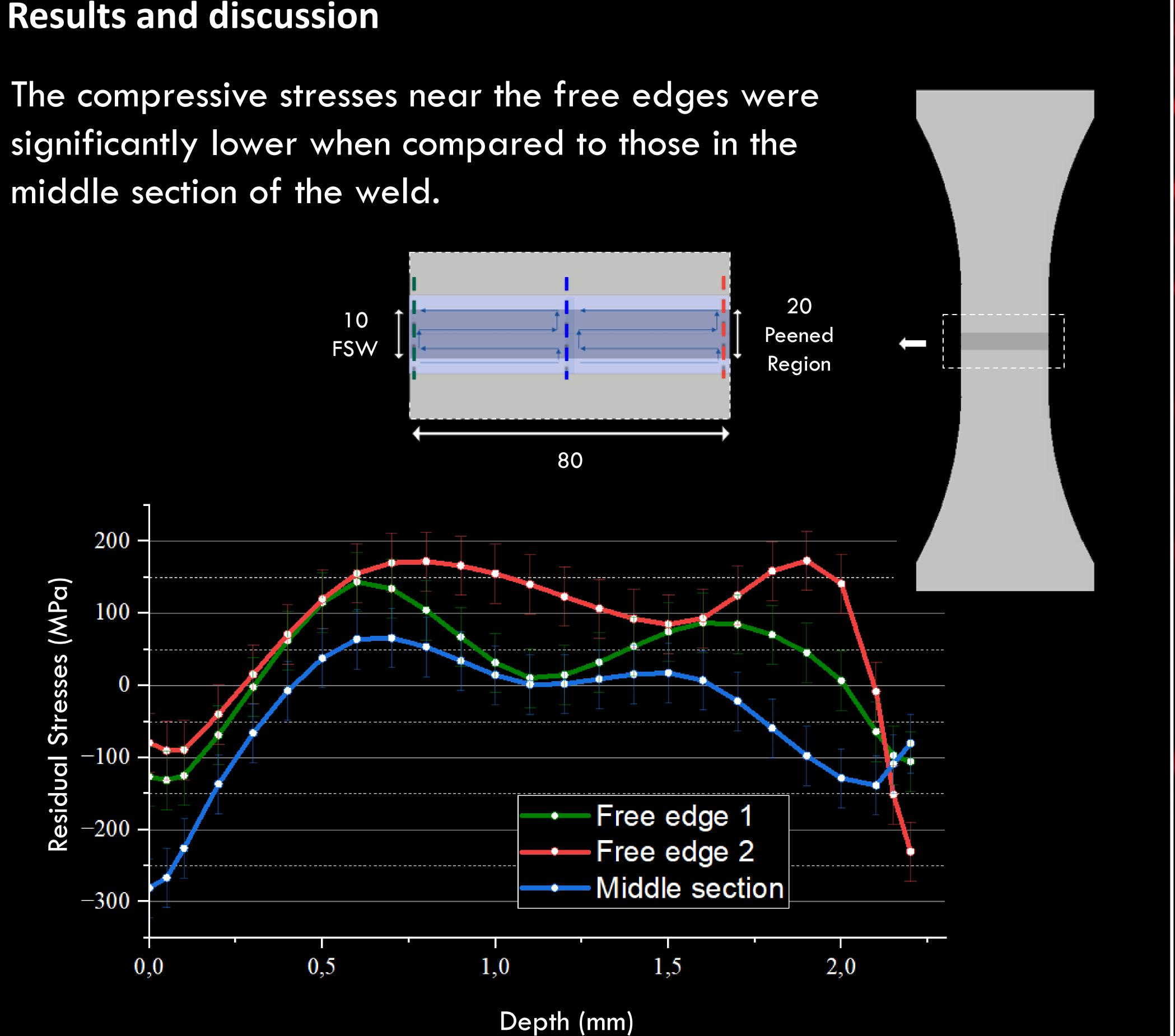
When peening next to a free edge, there is less material available for constraining the deformation.
